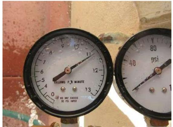
Water Pressure/Flow: Water pressure registered at about 40 psi at three different hose bibs.
